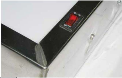
Simple On-Off Switch Impossible to create the desired luminance according to density of the developed x-ray film
