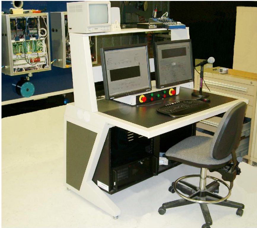
3in. High Accessory Garage located below LCD screens computer console cabinet was supplied with 19in EIA Equipment Racks
