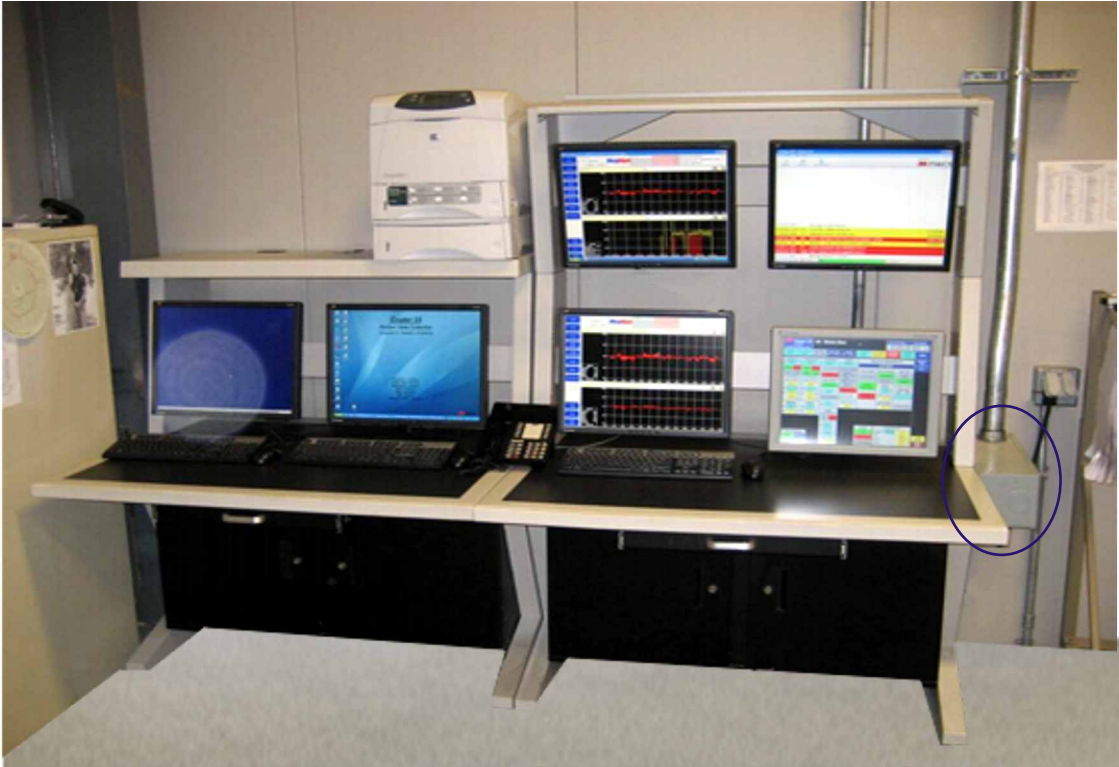
Left end unit is a catalog number AG-48D-1ERS-DMS A 48in wide Desk Console with 1-Tier Equipment Riser Shelf and Dual Monitor Supports
